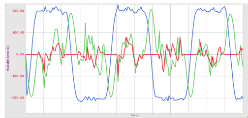
Fig. 8. The speed curve of the timing belt in three directions
