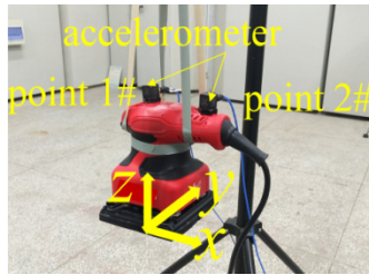
Fig. 3. The experiment to measure the acceleration of the housing
