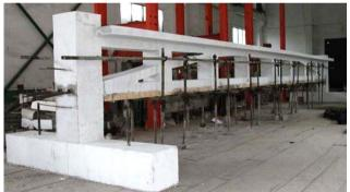
Fig. 3. Typical photo view of the APT specimen
