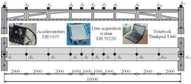
Fig. 4. Monitoring system and accelerometer location (mm)
