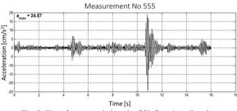
Fig. 2. Waveform recorded on the fifth floor in z direction
