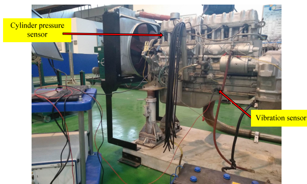
Fig. 3. Measuring position of vibration sensor
