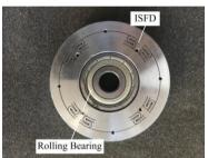
Fig. 2. ISFD with ball bearing
