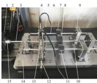
Fig. 5. Multiple parallel gear shafts test rig: 1 – motor, 2 – photoelectric sensor, 3 – drive shaft, 4 –acceleration sensor 1, 5 – acceleration sensor 2, 6 – driven shaft 2, 7 – driven gear 2, 8 – drive gear, 9 – ISFD elastic damping support, 10 – driven shaft 1, 11 – driven gear 1, 12 – acceleration sensor 3, 13 –acceleration sensor 4, 14 – base plate, 15 – coupling
