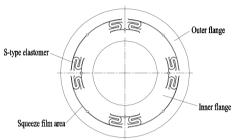
Fig. 1. Integral squeeze film damper
