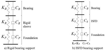
Fig. 3. Mechanical models of rigid bearing support system and ISFD bearing support system
