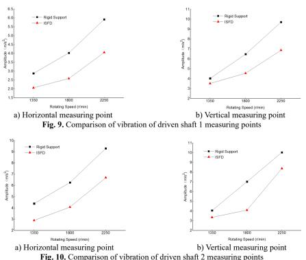
As shown in Fig. 9 and 10, the vibration of the gear shaft increases with an increase of the rotational speed. From the rigid support to the ISFD elastic damping support, the vibration amplitudes of the measuring points are greatly reduced. The experimental results show that the ISFD elastic damping support can make the multiple parallel gear shafts operate smoothly in a wide speed range.
