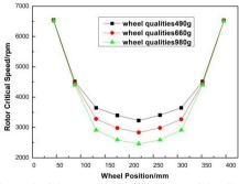
Fig. 4. The critical speed of the rotor with the change of the disc mass and position
