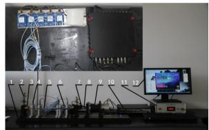
Fig. 1. Rotor critical speed measurement experimental device: 1 – the experiment pedestal, 2 – oiler, 3 – supporting bearing, 4 – eddy current displacement sensor and support, 5 – spindle, 6 – displacement sensor preamplifier, 7 – speed sensor, 8 – coupling, 9 – electric motor, 10 – vibration data analyzer, 11 – velometer, 12 – computer screen
