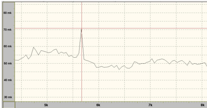
Fig. 8. Section of the spectrogram of natural oscillations corresponding to the middle pavement layer of the investigated road structure
