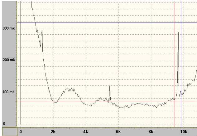
Fig. 11. Spectrogram of natural pavement oscillations for the “observation point” No. 204. The amplitude is 245 \mu\text{V} , the frequency \approx 9.8 \text{ kHz}
