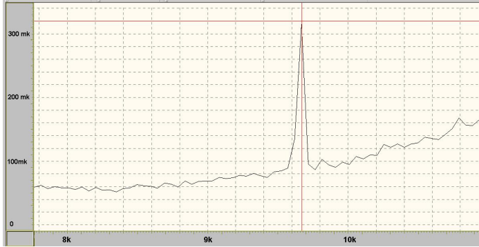
Fig. 7. Section of the spectrogram of natural oscillations corresponding to the upper pavement layer of the investigated road structure
