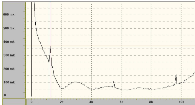
Fig. 6. Complex spectrogram of all self-induced vibrations of a particular road pavement sample. The spectrogram was obtained by georadar vibration-acoustic method
