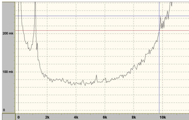
Fig. 9. Spectrogram of natural pavement oscillations for the “observation point” No. 212. The amplitude is 38 \mu\text{V} , the frequency \approx 9.8 \text{ kHz}
