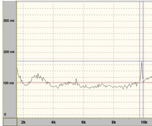
Fig. 10. Spectrogram of natural pavement oscillations for the “observation point” No. 208. The amplitude is 69 \mu\text{V} , the frequency \approx 9.8 \text{ kHz}
