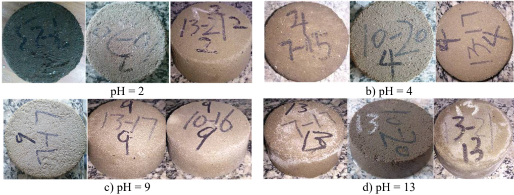
Fig. 15. The surface damage of specimens with different cement content in different environment
