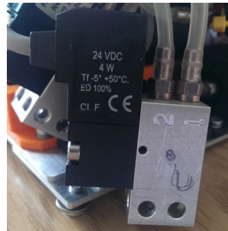
Fig. 12. Fuel cell stack valve
