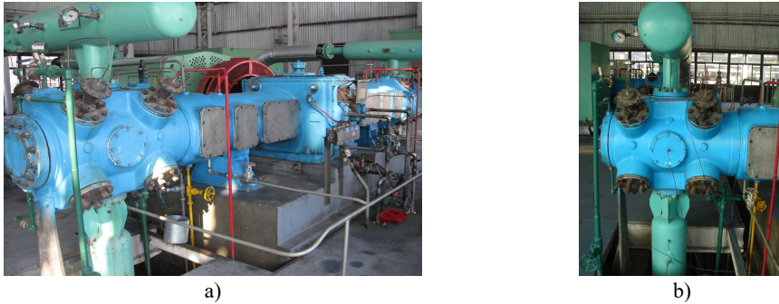
Fig. 4. Two-stage double-acting reciprocating compressor of 2D12 type
