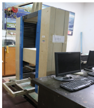
Fig. 2. RYL-600 rock shear rheometer test machine
