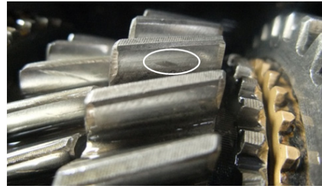
Fig. 3. Fault part of gear
