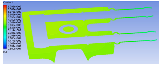
Fig. 13. Section temperature of sealing area without cooling water
