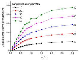
Fig. 9. The relationship between bond strength ratio and peak strength for different tangential bonding strength
