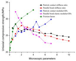
Fig. 4. Influence of the microscopic parameters on uniaxial compressive strength
