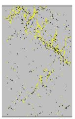
Fig. 7. Uniaxial compression failure crack (mainly tangential failure)
