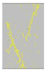
**Fig. 6.** Uniaxial compression failure crack (mainly normal failure)
