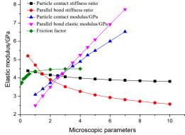
Fig. 2. Influence of microscopic parameters on elastic modulus
