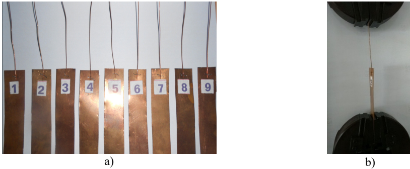
Fig. 13. a) Welded specimens, b) tensile testing of the weld specimen
