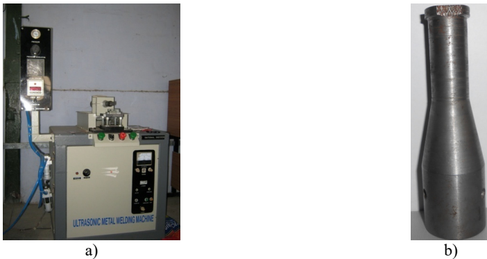
Fig. 12. a) Experimental setup, b) type II sonotrode
