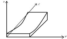
Fig. 1. Rectangular plate with one dimensional circular variation
