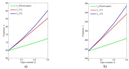
Fig. 5. Comparison of frequency modes with [11, 12] corresponding to taper constant  $(\beta)$
