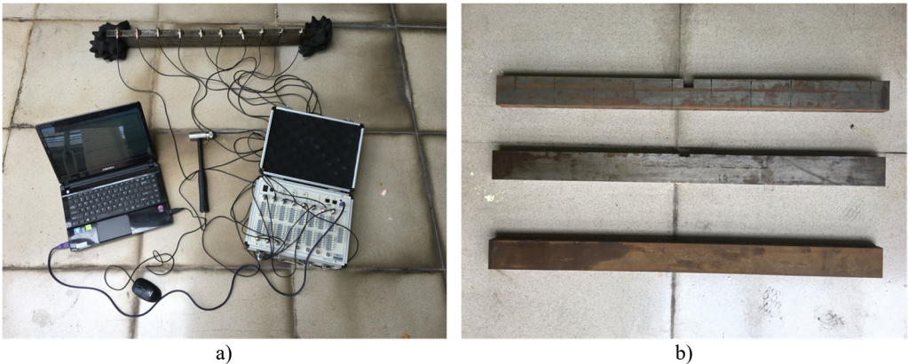
Fig. 3. Experimental set-up for modal analyses and testing specimens
