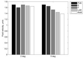
Fig. 5. Fluid velocity in healthy nucleus pulposus: PBL – pure  $10^{\circ}$  lateral bending, E – lateral bending + extension; F – lateral bending + flexion; LAR and RAR – lateral bending + axial rotation to the left or right
