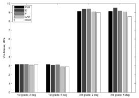
**Fig. 3.** Von Misses stress values induced by pure lateral bending and additional loads of 2° and 5° in healthy (1st grade) and degenerated (3rd grade) discs: PBL – pure 10° lateral bending, *E* – lateral bending + extension; *F* – lateral bending + flexion; LAR and RAR – lateral bending + axial rotation to the left or right
