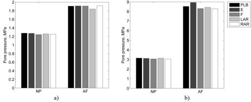
**Fig. 4.** Pore pressure comparison between loading cases: a) healthy intervertebral disc; b) degenerated intervertebral disc (PBL – pure  $10^{\circ}$  lateral bending, E – lateral bending  $+ 2^{\circ}$  extension; F – lateral bending  $+ 2^{\circ}$  flexion; LAR and RAR – lateral bending  $+ 2^{\circ}$  axial rotation to the left or right)
