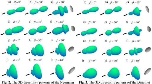
Fig. 2. The 3D directivity patterns of the Neumann boundary for Bessel half-cone angles  $\beta = 0^{\circ}$ , 30° and 60° at  $kr_0 = 5$ : a)-c) a/b = 1/3, d)-f) a/b = 1/2, g)-i) a/b = 2/1, j)-l) a/b = 3/1
