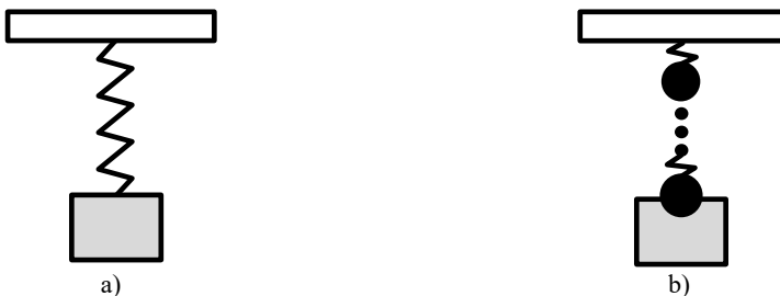
Fig. 2. The unit cell model of the different method: a) traditional transfer matrix method, b) the transfer matrix method for considering a distributed spring constant
