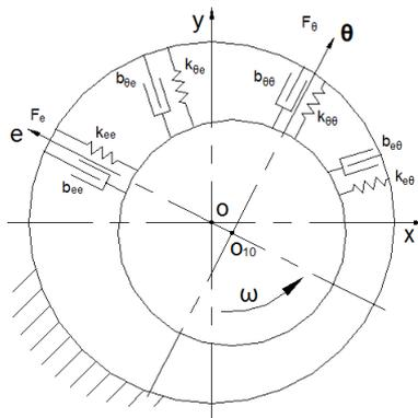
Fig. 2. Mechanical model of Tc bearing
