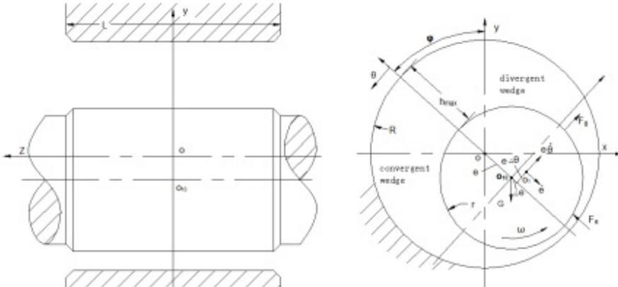
Fig. 1. The coordinate system of hydrodynamic equation and dynamic force diagram of Tc bearing
