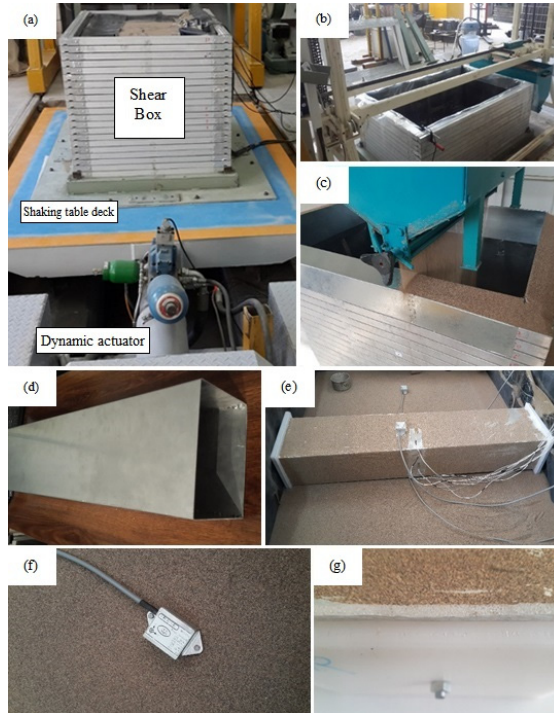
Fig. 1. a) University of Tabriz shaking Table, b) shear box and sand pluviation device, c) sand pouring, d) aluminum tunnel model, e) model preparation, f) 0.01 g accelerometer, g) Teflon plate and EPE foam
