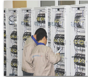
Over one thousand channels applied to paralleled synchronous hi-speed data acquisition of hypersonic wind tunnel
