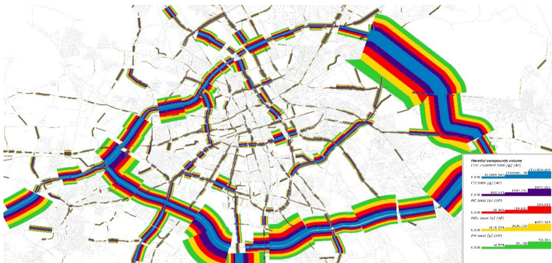
Fig. 9. Emission of pollutants for the traffic distribution in third scenario. Source: MTAW 2015 in PTV VISUM
