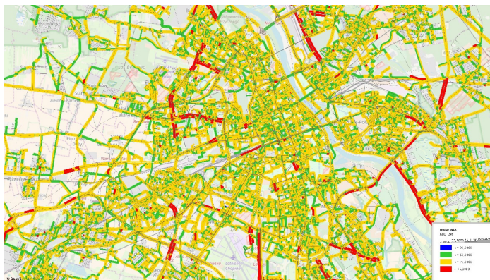
Fig. 10. Noise level for the traffic distribution in third scenario. Source: MTAW 2015 in PTV VISUM
