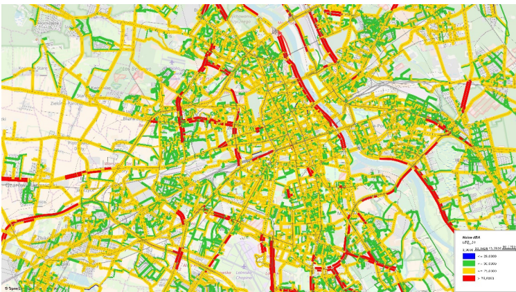
Fig. 7. Noise level for the traffic distribution in second scenario. Source: MTAW 2015 in PTV VISUM
