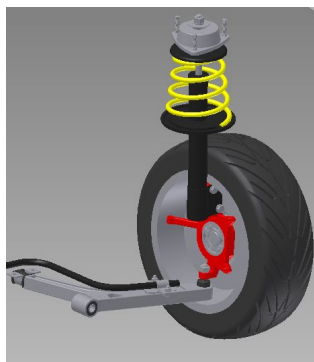
Fig. 1. Conventional independent suspension – McPherson strut
