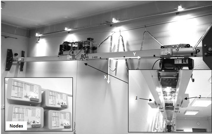
Fig. 3. Test stand and measurement nodes location, 1, two measurement nodes for measuring girder acceleration
