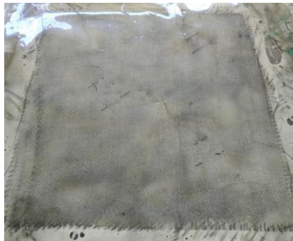
Fig. 3. Specimen containing 7 % MWNT's for [0^\circ/90^\circ] orientation
