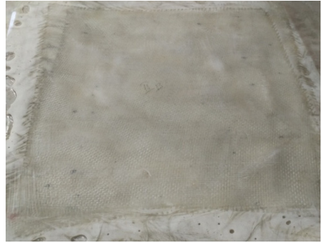
Fig. 2. Specimen containing 1 % MWNT's for [0^\circ/90^\circ] orientation
