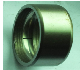
Fig. 3. The artificial spall of outer race (0.5 mm)
