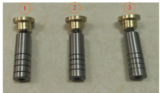
Fig. 3. Failure plunger: 1) plunger wear 0.2 mm 2) plunger wear 0.3 mm, 3 plunger wear 0.5 mm
