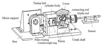
Fig. 2. Shaking table structure
