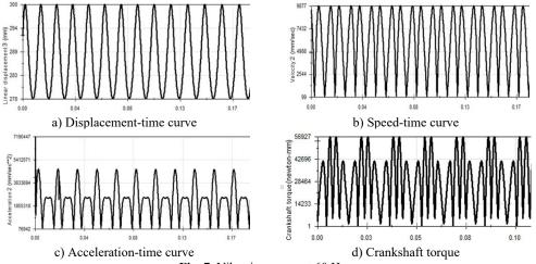
Fig. 7. Vibration curve at 60 Hz
