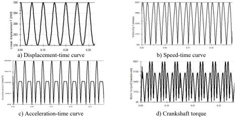
Fig. 6. Vibration curve at 20 Hz
