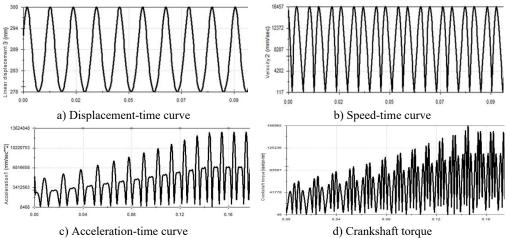
Fig. 8. Vibration curve at 100 Hz
