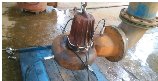
Fig. 16. Pressure sensors installed in the test pump
