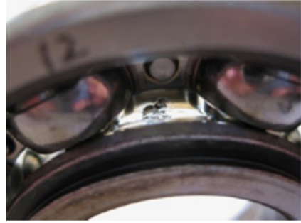
Fig. 14. The inner race fault
