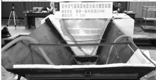
c) Experimental model Fig. 4. Shaking table test
