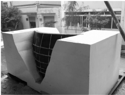
a) Organic glass supporting structure on the upstream face of dam
