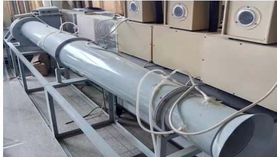
Fig. 1. Experimental platform for mechanical fault diagnosis of Centrifugal fan
