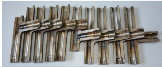
Fig. 11. The T-pipe after cutting
