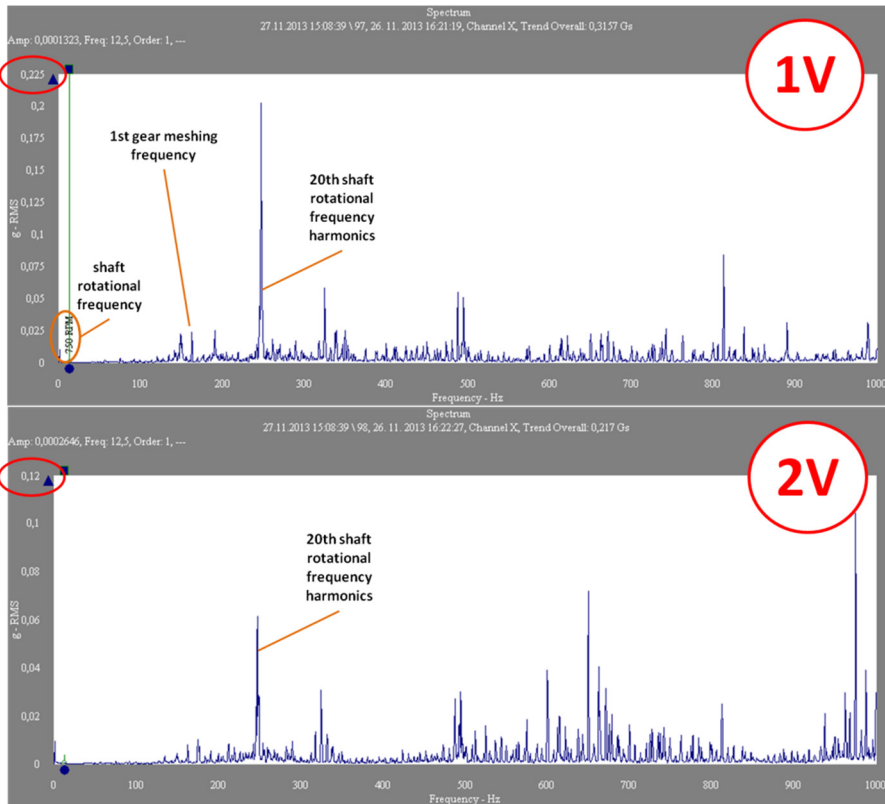
Fig. 3. The vibration specter – 1 V, 2 V – after repair
