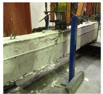
Fig. 8. New model's cracks (ultimate shear capacity)
