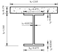
Fig. 3. Section sizes of the composite beam (unit: m)
