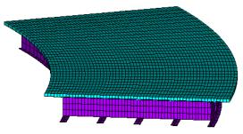
Fig. 7. Five-beam composite curved bridge model
