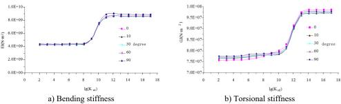
Fig. 4. Effective stiffness of the composite beam
