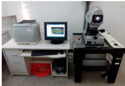
Fig. 8. NT1100 grating surface roughness measuring instrument
