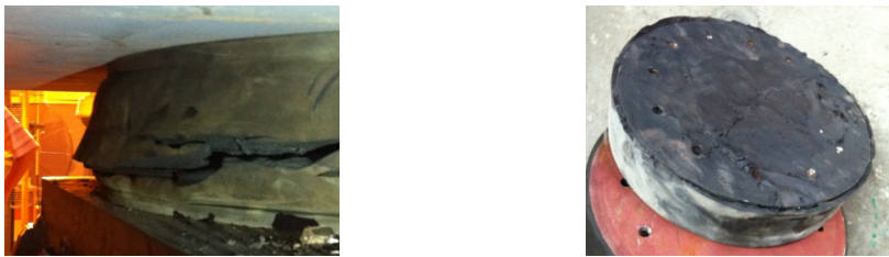
a) Rubber bearing layer ruptured (S-3) b) Rupture surface of shear failure (S-3)
