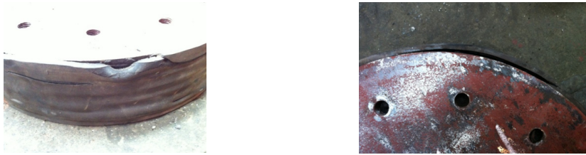
a) Protective rubber layer separated from the body b) Protective rubber layer striped
