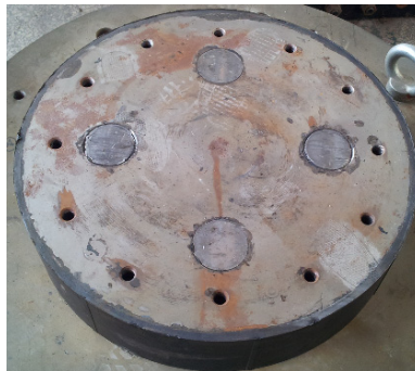
Fig. 3. Lead rubber bearing in the test
