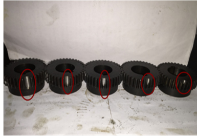
Fig. 12. Tooth broken fault of four different degree
