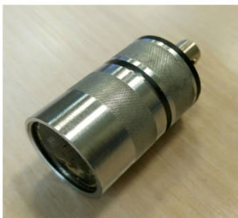
Fig. 5. Prototype of EMAT transducer designed for robotic crawler application
