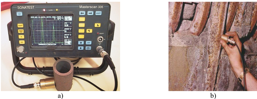
Fig. 3. a) EMAT transducer coupled with a popular standard UT instrument MS335 and b) the manual EMAT thickness measurement performed on boiler tubes
