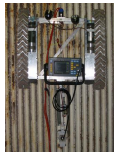
Fig. 6. Magnetic crawler for EMAT
