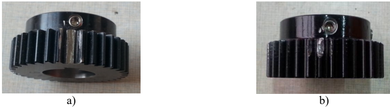
Fig. 8. Photos of faulty gear Z_3 : a) missing a tooth; b) a chipped tooth
