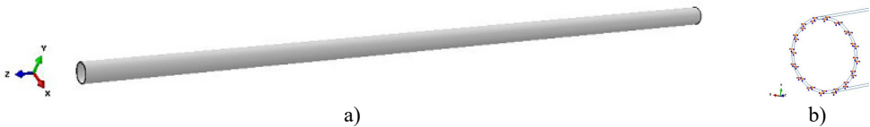
Fig. 9. a) A finite element model of the pipe was created using ABAQUS software, b) The boundary conditions for the experimental test
