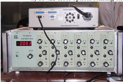
b) Dynamic resistance strain gauge and data acquisition instrument for measuring the change of top tension
