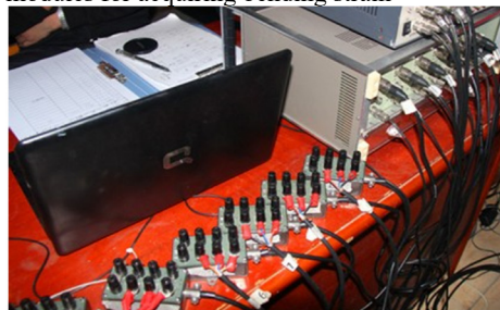
b) Dynamic resistance strain gauge and data acquisition instrument for measuring the change of top tension
