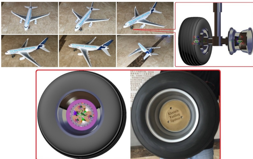
Fig. 2. The virtual prototype and scaled model of the powered wheel
