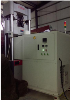
Fig. 5. a) Universal testing machine equipped with a temperature control box in which the dynamic mechanical parameters of the soft pads in b) WJ-7 fasteners are measured under -60 to +20 °C
