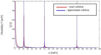
**Fig. 1.** Absolute values of dynamical flexibility of the beam with combination of boundary conditions (*F*) and (*P*), for n = 1, 2, 3
