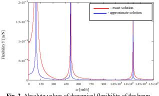
**Fig. 2.** Absolute values of dynamical flexibility of the beam with combination of boundary conditions (*C*) and (*S*), for n = 1, 2, 3
