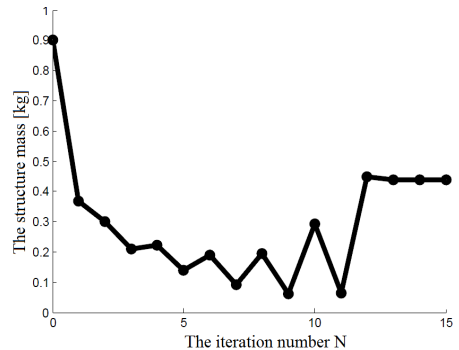
Fig. 28. The iteration history of structure mass
